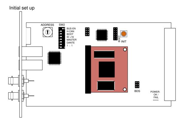
**ADDRESS:** This **rotary encoder** sets the **CAN ID** of the **C8315**. The switch positions are
