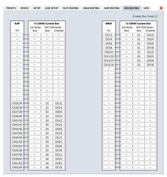
This pane shows the possible sources for the c8k busses from the AoIP as well as from the MADI interfaces. The above example is the result of the **FAST ROUTING** settings above.
