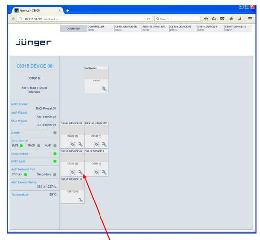
By clicking on the spanner tool symbol you will be forwarded to the control pages of the **C8315** and the status pane on the left hand side, which is also shown on mouse over.
