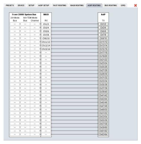
This pane shows the possible sources for the AoIP interface. The above example is the result of the **FAST ROUTING** settings above.
