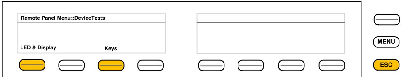
Pressing **<LED & Display>** lets you check the bar graph and status LEDs basic colors:
