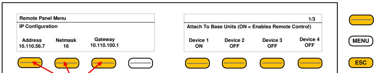
You may press the respective **<F-Keys>** and a separate window will appear for comfortable set-up of the respective part of the IP configuration.
