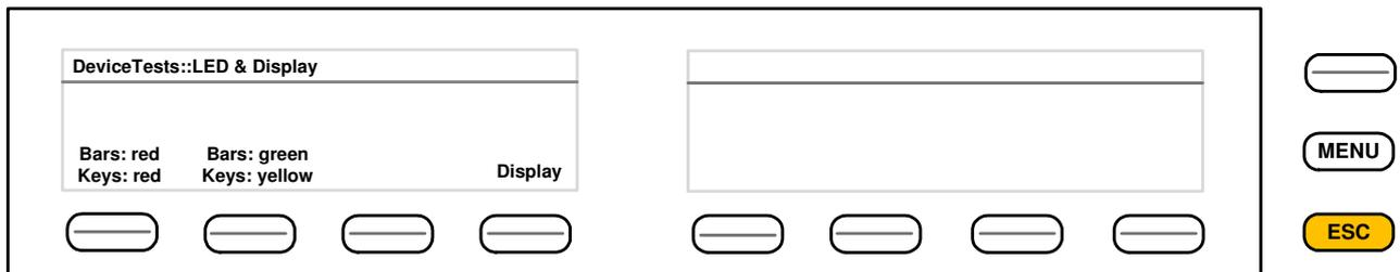
All bar graph and key LEDs must light in the respective color. Pressing the **<Display>** button will turn on both display windows in amber color. You will return by pressing the **<ESC>** button.
