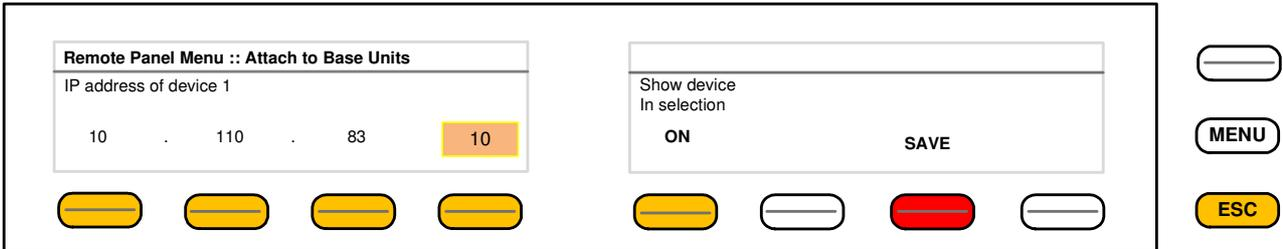
Same procedure: Set up the IP address of the device you are about to attach. You must turn "Show device in selection" to ON in order to reach that device via the initial display later on. Pressing <SAVE> will return to the "Remote Panel Menu" menu page 1/3.
