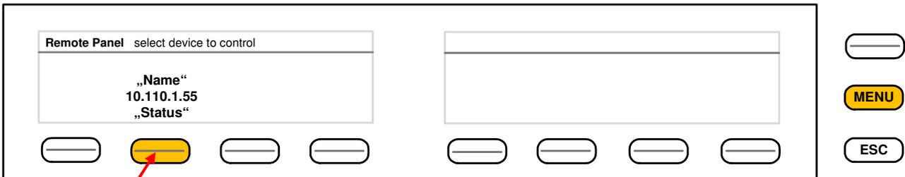
If you press the **<F-Key>** the X\*AP RM<sub>1</sub> remote panel will connect with that unit. (The above example has just one unit attached for remote control). Now the X\*AP RM<sub>1</sub> remote panel will gather all necessary information from that unit (it may take a few seconds) and open up the **main display**:
