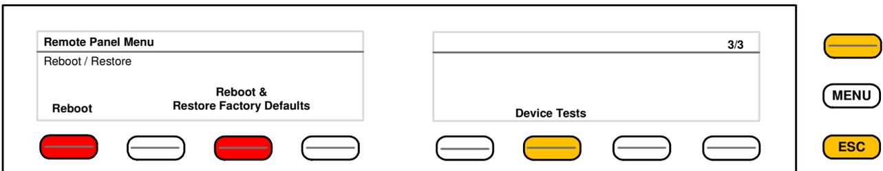
Page three allows you to reboot or restore of factory defaults. It also offers testing the device. X\*AP RM<sub>1</sub> remote panel LEDs, buttons and the rotary knob. Pressing the Device Test button opens up further menus to test the respective items.
