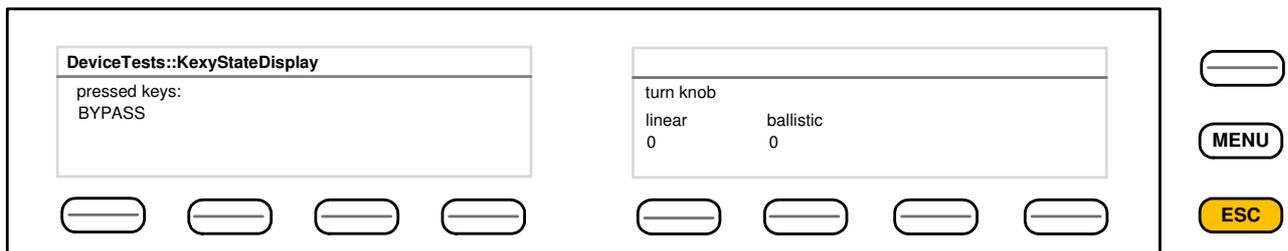
When you press a key of your choice the name of it will be displayed - in the example above, the **<BYPASS>** button. You can also check the rotary encoder by either turning the knob or pressing on it. If you turn the knob you will see the momentary value generated in linear and ballistic values. Pressing on the knob will show the name **ENTER** in the left display.
