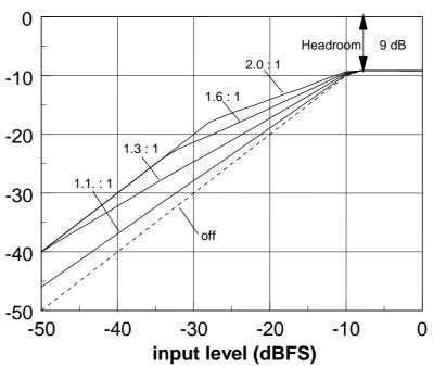
compression gain: max. 10 dB parameter: ratio
