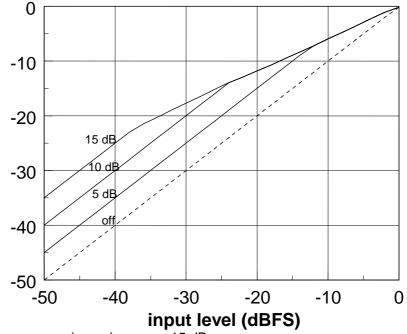
compression gain: max. 15 dB parameter: compression gain
