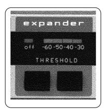
The expander **THRESHOLD** can be changed upward or downward with two buttons and is visible on the LEDs above them. Four expander thresholds (-60 dB, -50 dB, -40 dB, -30 dB) can be selected. The threshold level is related to the choosed digital reference level.
