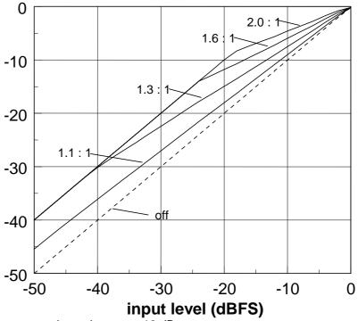
compression gain: max. 10 dB parameter: ratio
