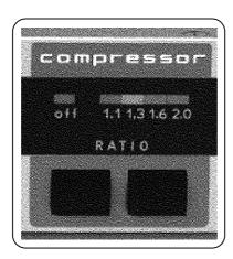
The compression ratio is adjusted by pressing the RATIO button and the currently selected ratio is shown by the lighting of the appropriate LED above the RATIO button.
