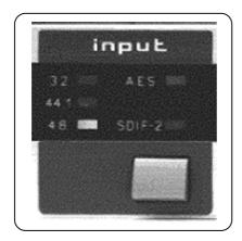
By pressing the button in the input section the required input signal can be selected. Each time the button is pressed the input selection is changed and one of the three LED's above the button lights **green** to show the newly selected input ( AES or SDIF-2 ).. If the LED lits **red** the input signal was recorded with **emphasis** or the deemphasis switch on the rear panel is on.
