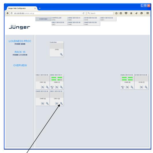
Clicking on the spanner tool within the module graphics of the C8631 will open the pages of that module.
