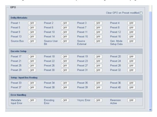
Clear GPO on Preset modified If a GPO indicates that a certain preset is loaded and if you change parameters which are related to that preset the word "modified" will be displayed in line with the preset name in the status window.
