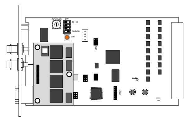
Set the **ADDRESS** rotary encoder to an address, which is not in use by another module of a C8000 frame (for details regarding CAN addressing, see C8k system manual).
