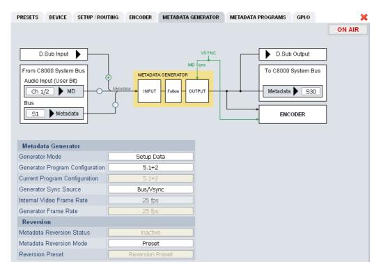
The **C8631** provides an extra metadata generator that can be used transparently (input metadata appear at the outputs) or controlled via the set-up data. In the latter case the output metadata may be derived selectively from the input.
