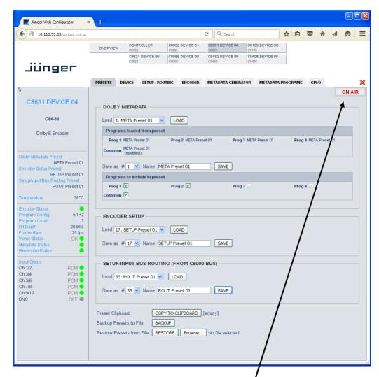
Important Note! The module may be controlled in ON AIR mode € I.e. all settings have immediate effect. While in OFF AIR mode you may prepare presets without affecting the current operation. In this case online functions like preset clip board are not available.
